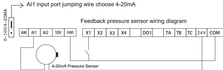
Remote pressure gauge wiring diagram
