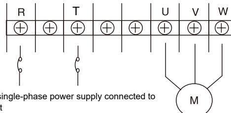
220V single-phase power supply connected to R and t
